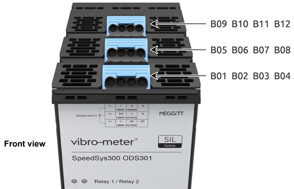
Figure 2-3: SpeedSys300 ODS301 module – top connector pinouts
