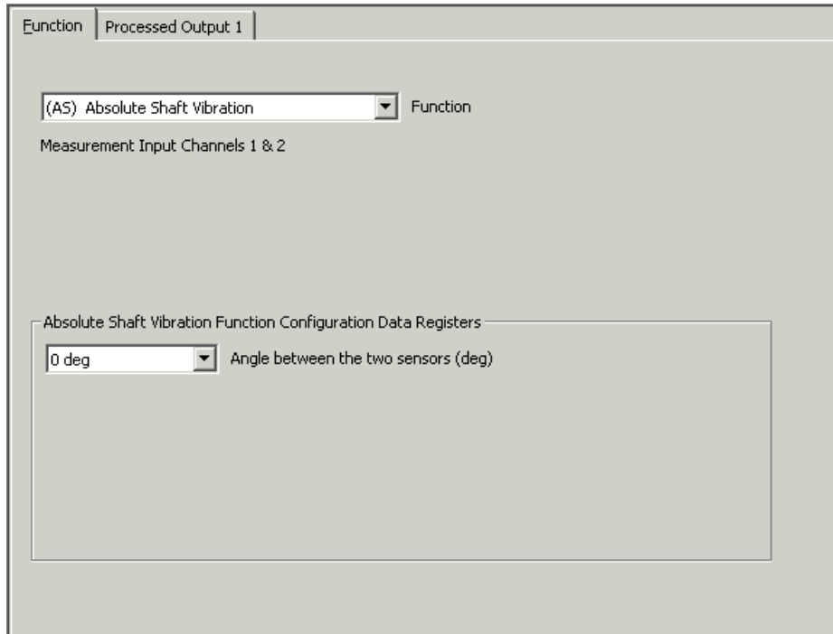
Figure 8-26: Typical “Function” tab for Absolute Shaft Vibration processing function
