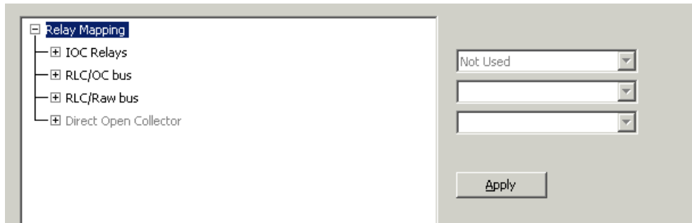
Figure 10-2: Relay Mapping tree structure (for MPC4 card)
