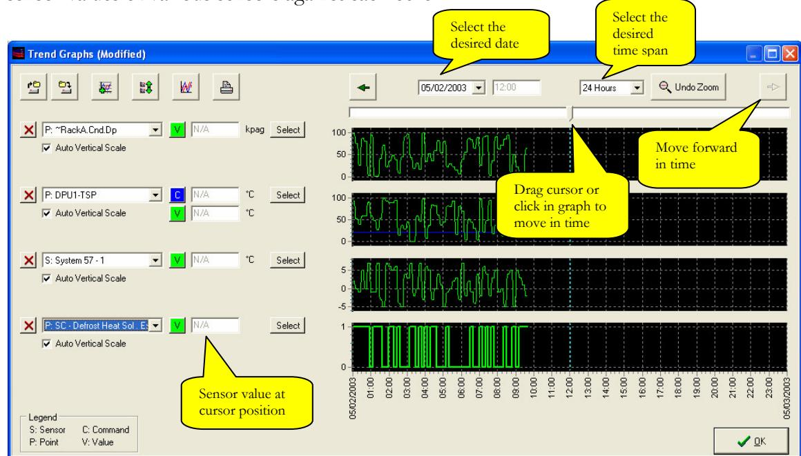
When adding or removing a graph, each graph is resized vertically so that all graphs fit in the windows. A maximum of 7 trend graphs can be used on the same screen.
