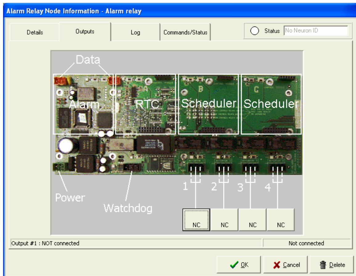
It shows you which outputs are free and which outputs are used. You will be able to assign alarm relays to these outputs only after you drop the alarm relays. Assignment is bi-directional. You can come here and click on the outputs to assign an alarm relay or you go on the relay to select the alarm relay node and output.
