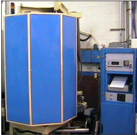
Figure 3 - A unique characteristic of Bayside manufacturing capabilities is our in-house plasma nitriding equipment.
