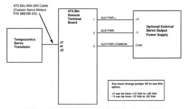
Figure 24-9. Optional Cable: External Power Supply for DC Servo Output with Remote Terminal Board
