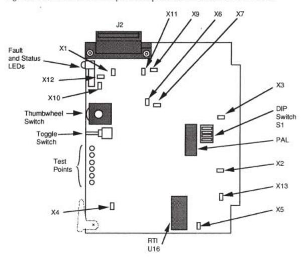
Figure 26-1. Model 473.66c Encoder Servo Translator Component Location
