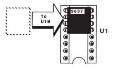
Figure D-2. U1B Position for External Interrogation
