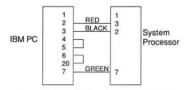
Figure 29-8. Cable Configuration (473.50c-25A-300)
