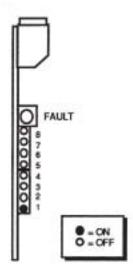
Figure 8-11. LEDs after Normal Power-up (Version 1 Firmware)
