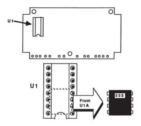
Figure D-1. U1A Position for Internal Interrogation
