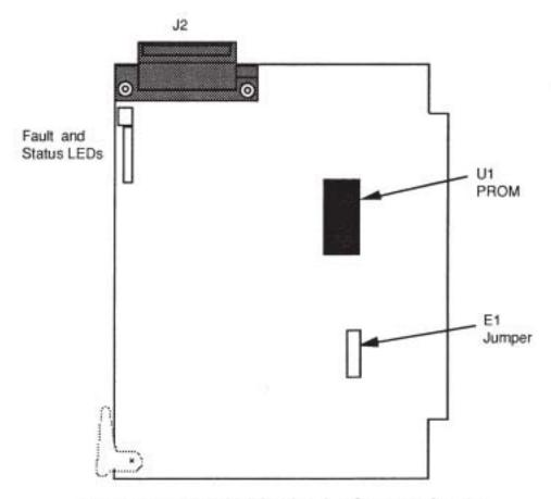
Figure 9-1. Model 473.04c RS232 Interface Component Location
