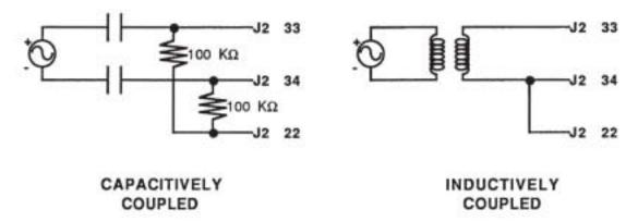
Figure 8-4. Providing a DC Path for Input Bias Currents (Channel 1)
