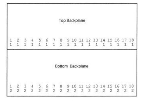
Figure 3-3. Card Labels and Slot Numbers.
