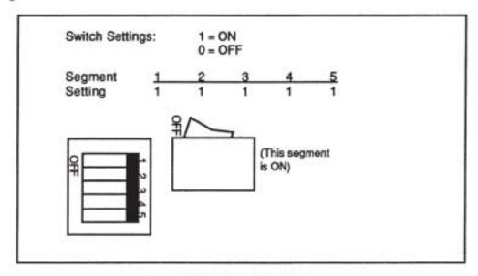
Figure 16-2. DIP Switch Setting
