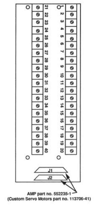
Figure 11-1. 473.38c-02A Remote Terminal Board
