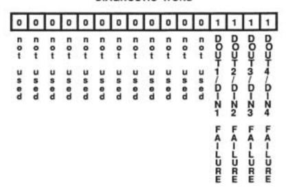
Figure 8-18. Diagnostic Word for the Digital Loop-back Test
