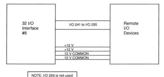
Figure 3-2. Remote Data Bus Configuration
