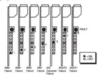
Figure 8-14. LED Indications for the Analog Loop-back Test
