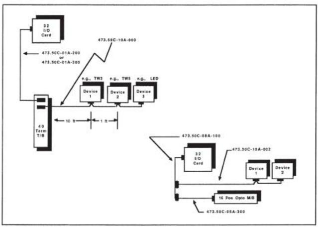
32 I/O to Remote Terminal Board and Remote Data Bus
