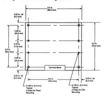
Figure 27-3. Mounting Dimensions
