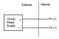
Figure 8-3A. External Power Supply for DC to DC Converter
