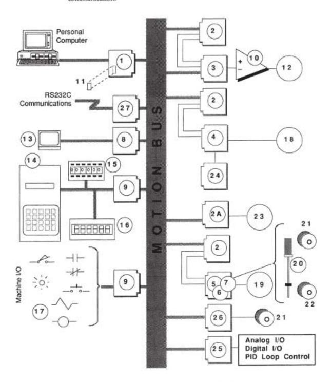
Figure 2-1. General Configuration of the Motion Plus/473 System
