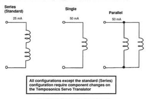
Figure 24-13. Servo Valve Configurations
