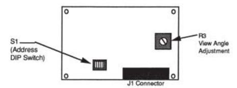
Figure 16-1. Model 473.13c Remote LCD Display Component Location
