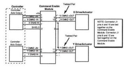
Figure 27-2. Cable Configurations
