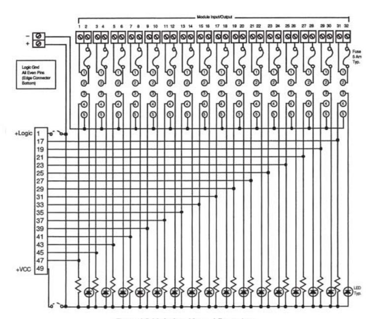
Figure 12-5. Motherboard Internal Connections
