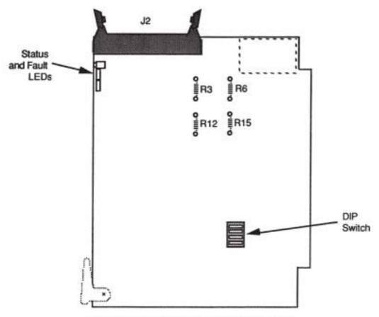
Figure 8-1. Model 473.70c Analog I/O Processor
