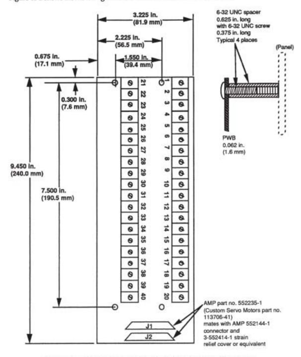
Figure 11-2. 473.38c-02A Remote Terminal Board Mounting Dimensions
