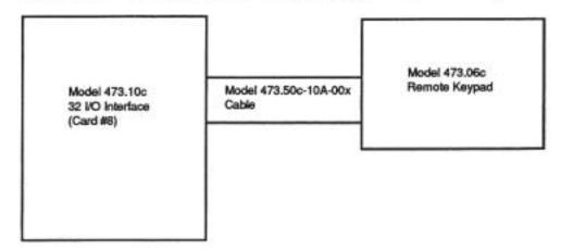
Figure 13-3. Cable Configuration for the Remote Keypad
