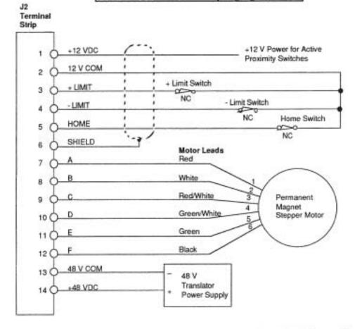
Figure 19-3. Typical Cabling Connections for the Model 473.20c Stepper Translator
