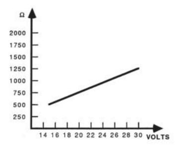
Figure 8-10. Maximum Load Resistance vs. Current Loop Power Supply Voltage.
