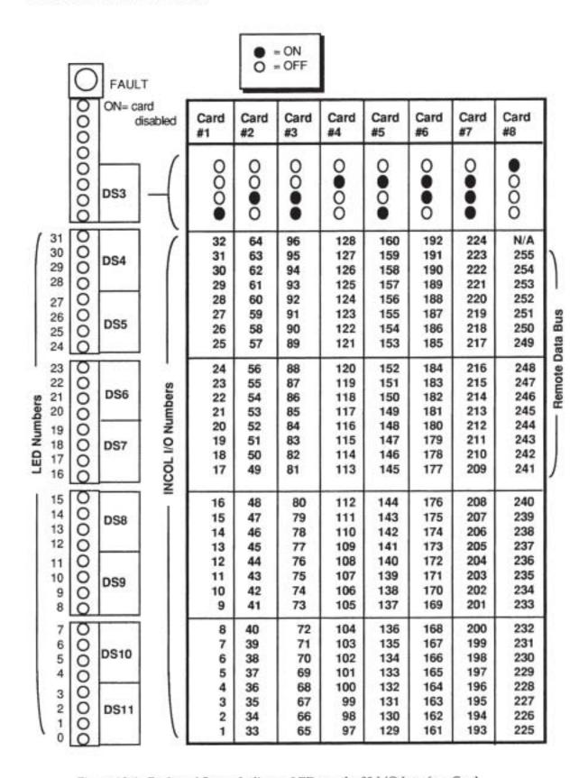
Figure 10-6. Fault and Status Indicator LEDs on the 32 I/O Interface Card
