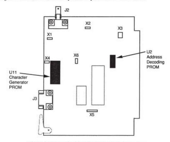
Figure 17-1. Model 473.08c CRT Interface Component Location
