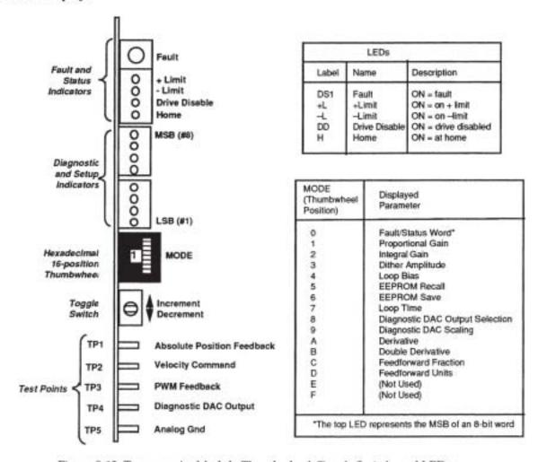
Figure 9-12. Temposonics Module Thumbwheel, Toggle Switch, and LEDs
