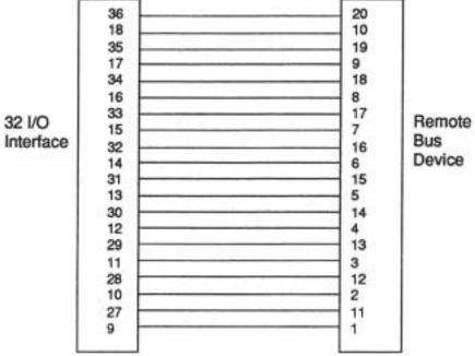
Figure 29-6. Cable Configuration (473.50c-10A-0XX Remote Data Bus Cable)
