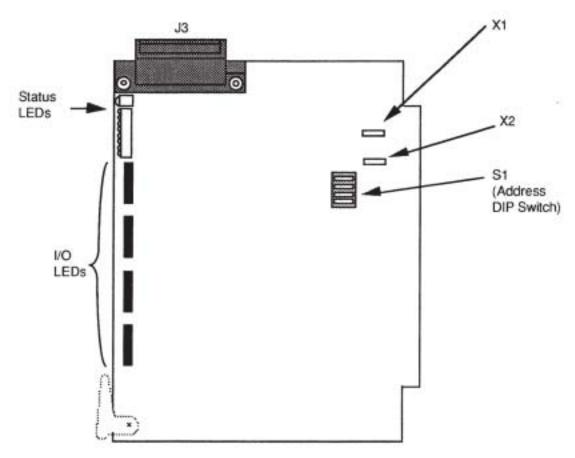
Figure 10-1. Model 473.10c 32 I/O Interface Component Location
