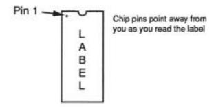
Plug pin 1 of the chip into pin 1 of the socket (pin 1 is in the upper left hand corner of the socket if you position the card with J2 facing up).
