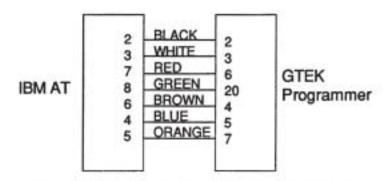
Figure 29-11. Cable Configurations (473.50c-26B-300)
