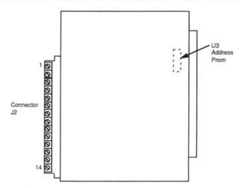
Figure 19-1. Model 473.20c Stepper Translator Component Location
