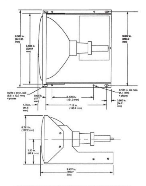
Figure 18-3. Mounting Dimensions, 9-inch CRT Display Monitor
