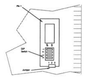
Set the jumper and the DIP switch on the Assembly as required. When the jumper is connected 2-3, it addresses any of the translators as follows:
