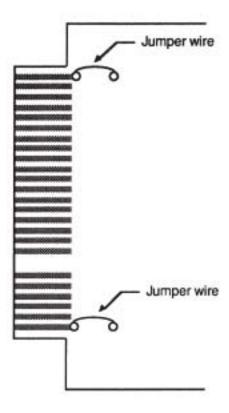
Figure 12-2. Jumpers on the 473.36c-02 Motherboard
