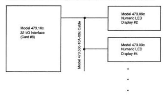
Figure 15-2. Cable Configuration for the Numeric LED Display
