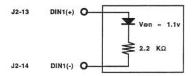
Figure 8-6. Equivalent Digital Input Circuitry.
