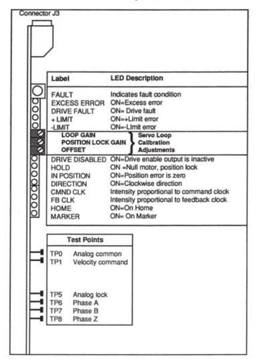
Figure 22-5. LEDs and Test Points
