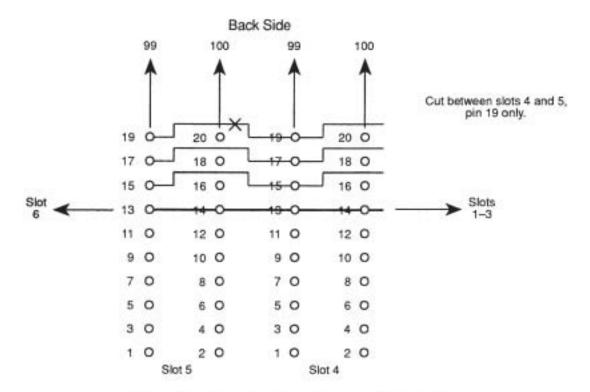
Figure 3-5a. Example of Cuts Between Slots 4 and 5
