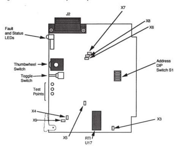
Figure 25-1. Model 473.65c Resolver Servo Translator Component Location
