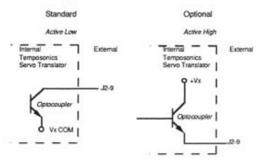
Figure 24-11. Enable Circuit Configurations Changing the Enable Sense
