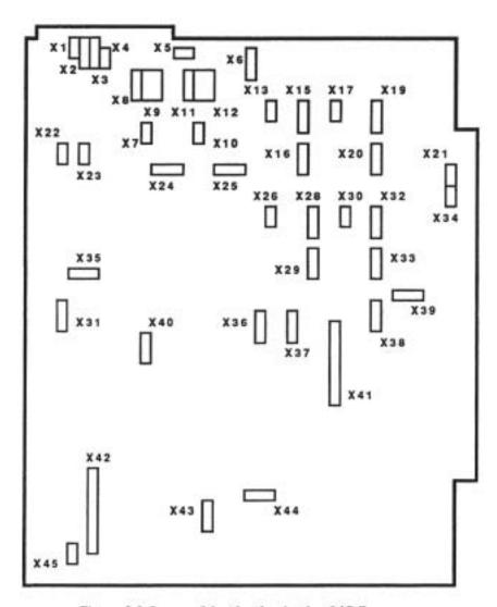
Figure 8-2. Jumper Map for the Analog I/O Processor
