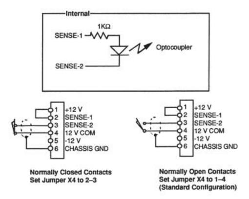
Figure 6-3. Sample Sensor Cables
