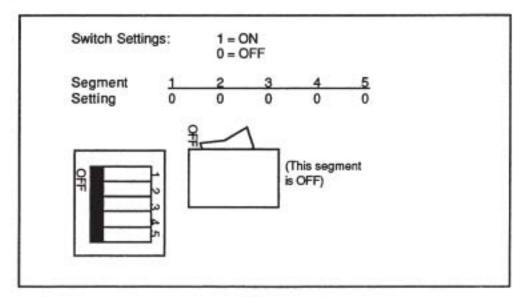
Figure 13-2. DIP Switch Setting
