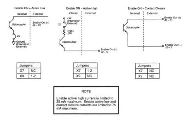
Figure 26-5. Enable Circuit Configurations Changing the Enable Sense
