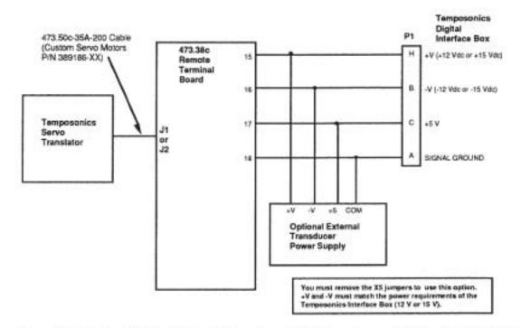
Figure 24-7. Optional Cable: External Power Supply for Transducer with Remote Terminal Board
