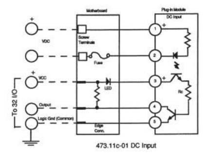
Figure 12-7. DC Input Module Internal Connections
