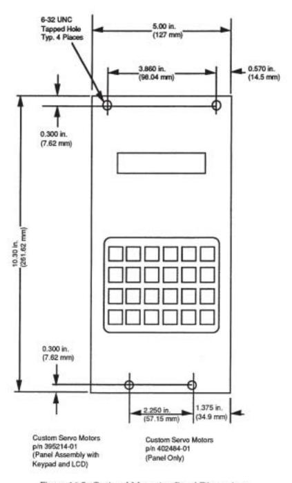
Figure 16-5. Optional Mounting Panel Dimensions
