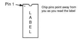
Plug pin 1 of the chip into pin 1 of the socket (pin 1 is in the upper left hand corner of the socket if you position the card with J2 facing up).
