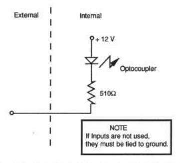
Figure 25-6. Internal Configuration of Limit, Home, and Drive Fault Inputs
