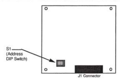
Figure 13-1. Model 473.06c Remote Keypad Component Location
