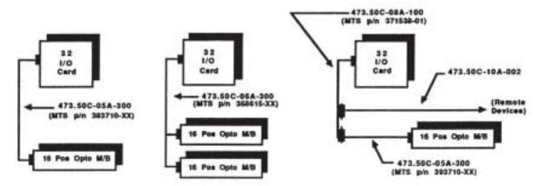
Figure 12-3. Cabling for the Motherboard
