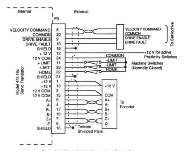
Figure 22-3. Direct Cabling Connections (Optional)
