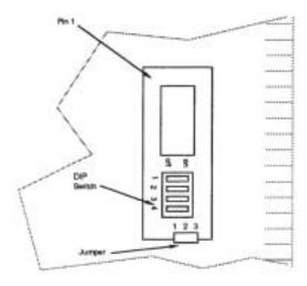
Set the jumper and the DIP switch on the Assembly as required. When the jumper is connected 2-3, it addresses any of the translators as follows:
