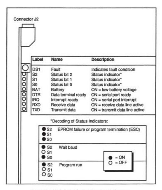
Figure 5-2. High Speed System Processor Indicators
