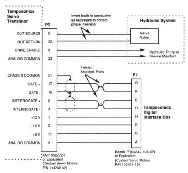
Figure 24-3. Optional Cabling Example When Using an Analog Current Velocity Command
