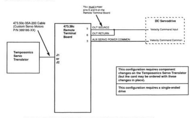
Figure 24-5. Optional Cable: Servo Drive with Remote Terminal Board
