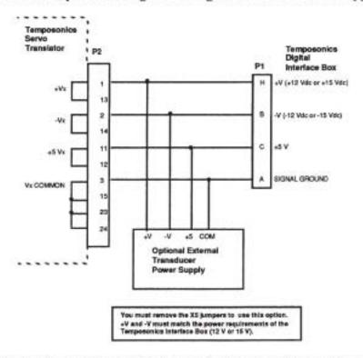
Figure 24-6. Optional Cable: External Power Supply for Transducer
