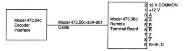
Figure 23-2. Cable Configuration for the Encoder Interface
