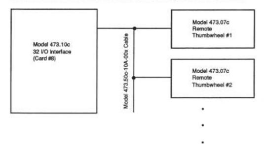
Figure 14-2. Cable Configuration for the Remote Thumbwheel
