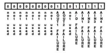
Figure 8-15. Diagnostic Word for the Analog Loop-back Test
