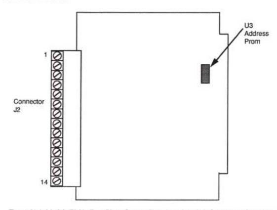
Figure 21-1. Model 473.23c Four-Phase Stepper Translator Interface Component Location
