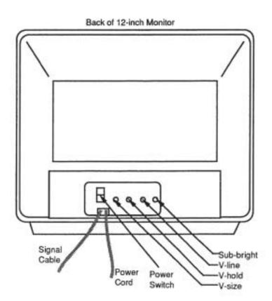
Figure 18-2. Model 473.91c-004 CRT Display Monitor Component Location (12-inch Monitor)
