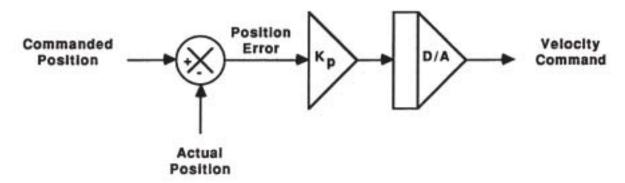
Figure A-8. Position Controller Functional Diagram
