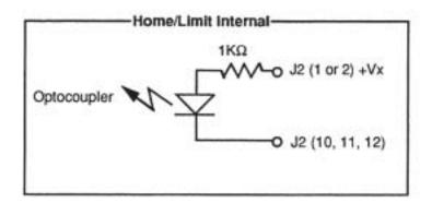
Figure 7-4. Home/Limit Inputs-Internal Configuration
