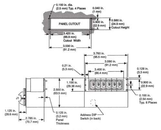
Figure 14-4. 473.07c Thumbwheel Mounting Dimensions
