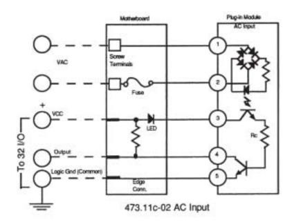
Figure 12-8. AC Input Module Internal Connections
