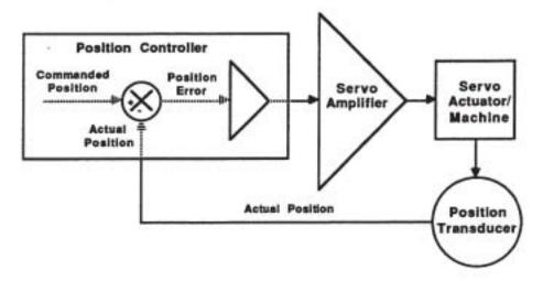
Figure A-2. Typical Position Loop
