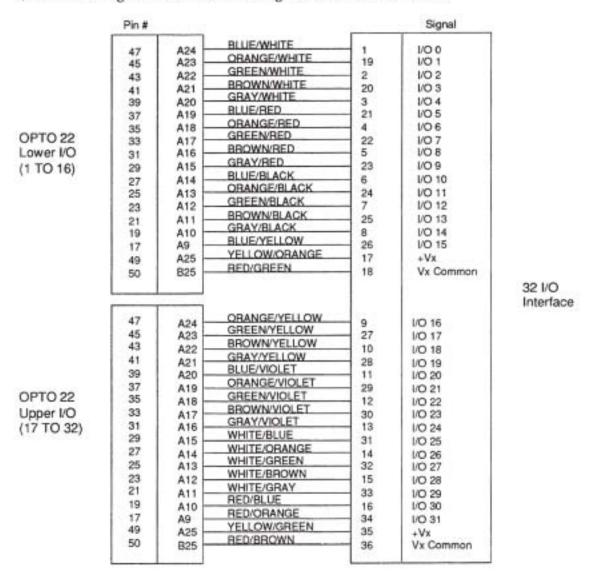
Figure 10-2b. Connecting 32 I/O Card to Two Opto Motherboards
