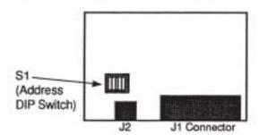
Figure 15-1. Model 473.09c Numeric LED Display Component Location
