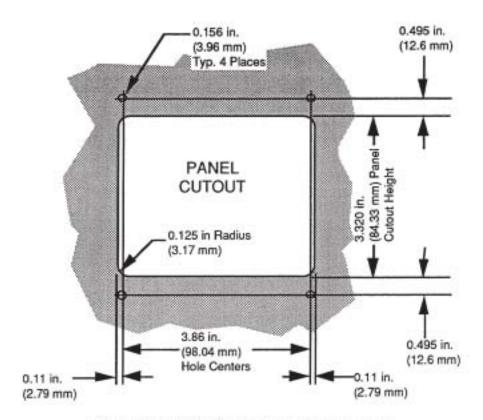
Figure 13-4. 473.06c Keypad Mounting Dimensions
