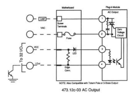
Figure 12-10. AC Output Module Internal Connections
