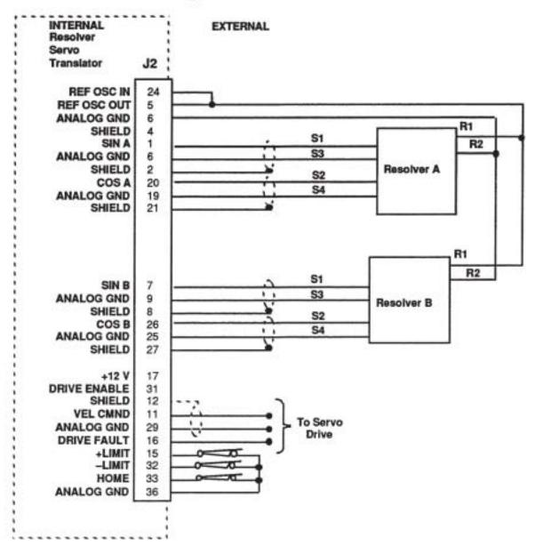
Figure 25-3. Wiring Example
