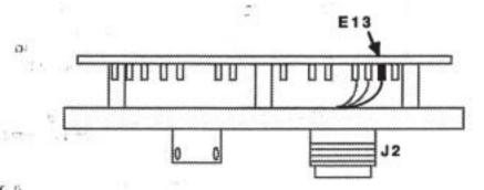
Figure D-5. DIB Internal Connection for Negative Pulse (Short) Transducer
