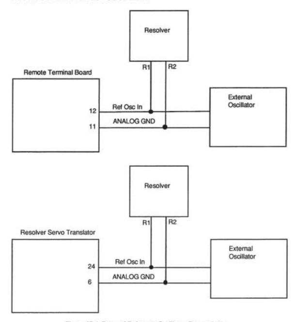
Figure 25-4. External Reference Oscillator Connections
