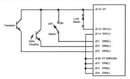
Figure 8-7. Examples of Digital Input Configurations.
