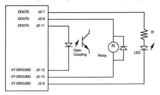
Figure 8-8. Examples of Digital Output Configurations
