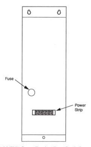
Figure 20-1. Model 473.31c Stepper Translator Power Supply Component Location
