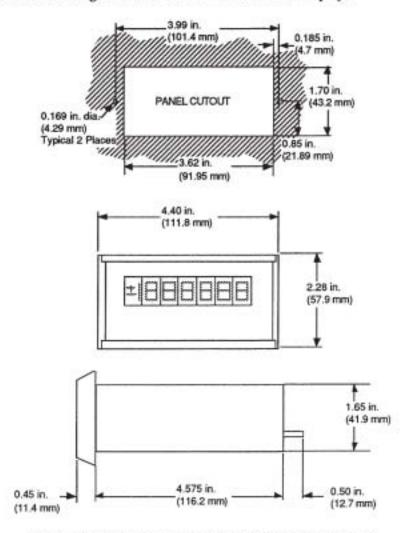
Figure 15-4. Numeric LED Display Mounting Dimensions
