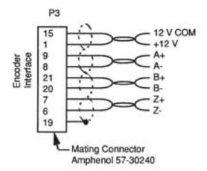
Figure 23-3. Wiring Example
