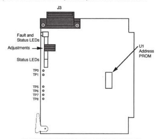
Figure 22-1. Model 473.19c Servo Translator Component Location
