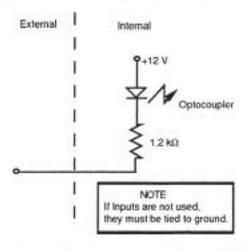
Figure 24-12. Internal Configuration of Limit and Home Inputs
