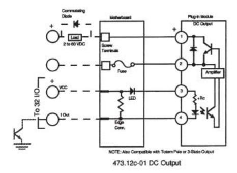
Figure 12-9. DC Output Module Internal Connections
