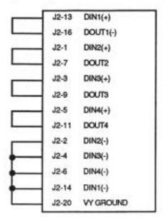
Figure 8-16. Connections for the Digital Loop-back Test
