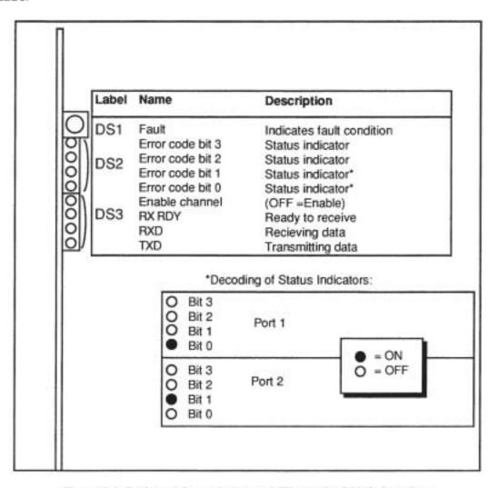
Figure 9-3. Fault and Status Indicator LEDs on the RS232 Interface
