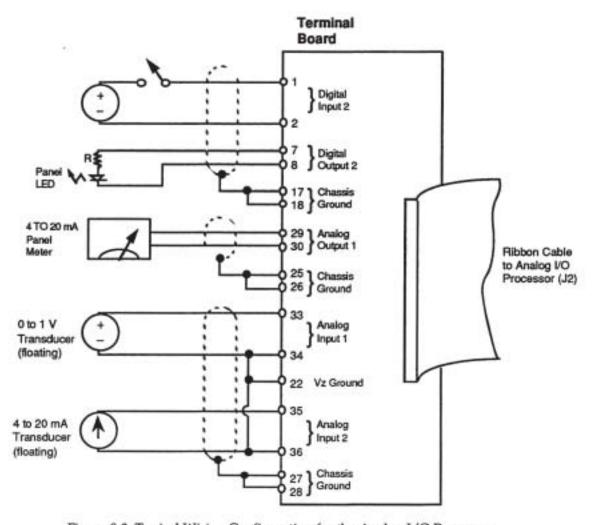
Figure 8-3. Typical Wiring Configuration for the Analog I/O Processor
