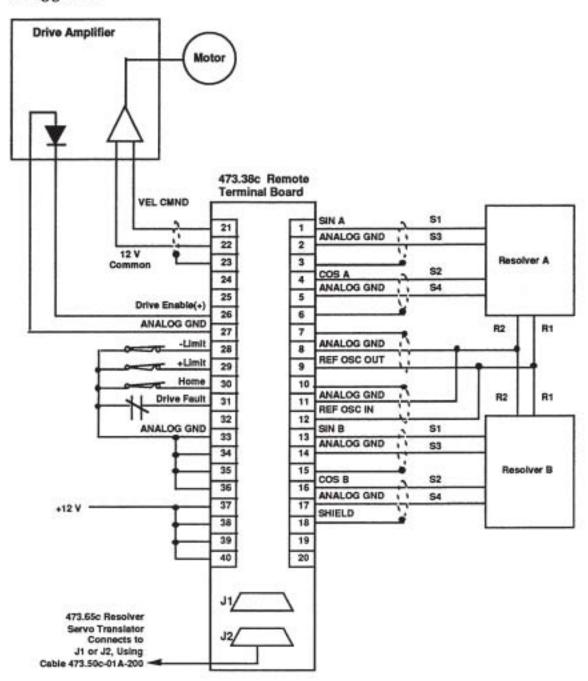
Figure 25-2. Cable Configuration for the Resolver Servo Translator
