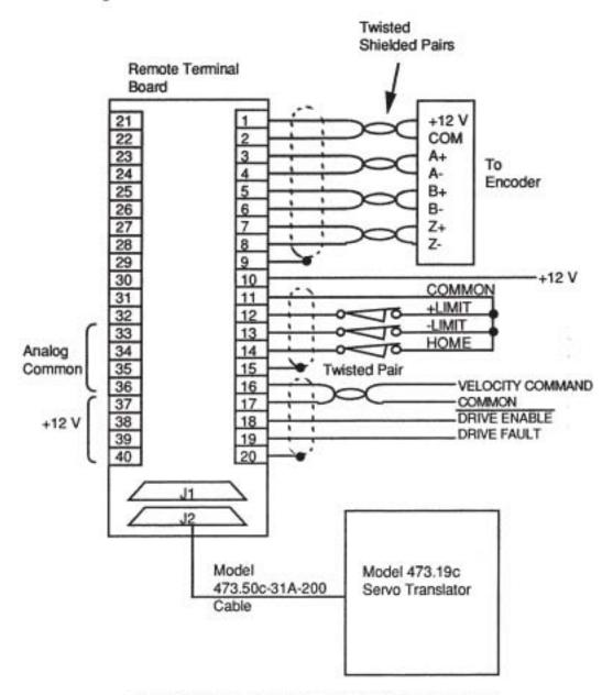
Figure 22-2. Cable Connections for the Servo Translator
