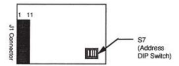
Figure 14-1. Model 473.07c Remote Thumbwheel Component Location
