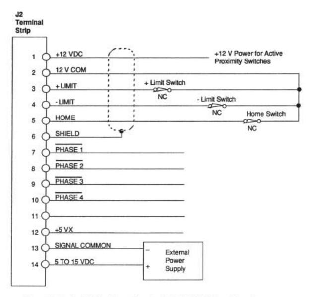
Figure 21-3. Typical Cabling Connections for the Model 473.23c Four-Phase Stepper Translator Interface
