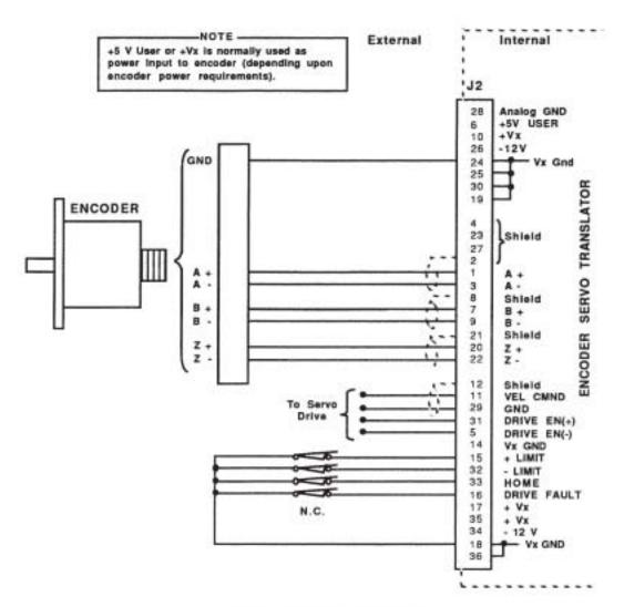
Figure 26-3. Wiring Example
