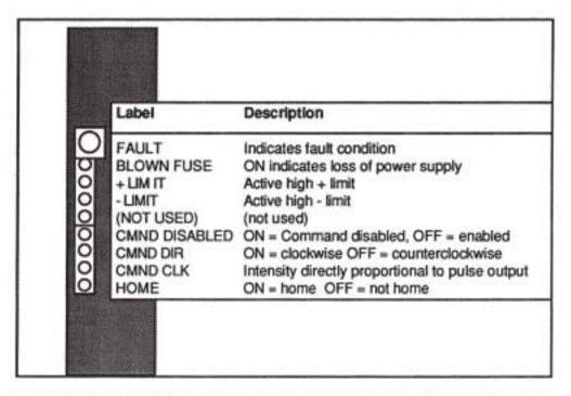
Figure 21-4. Fault and Status Indicator LEDs on the Four-Phase Stepper Translator Interface
