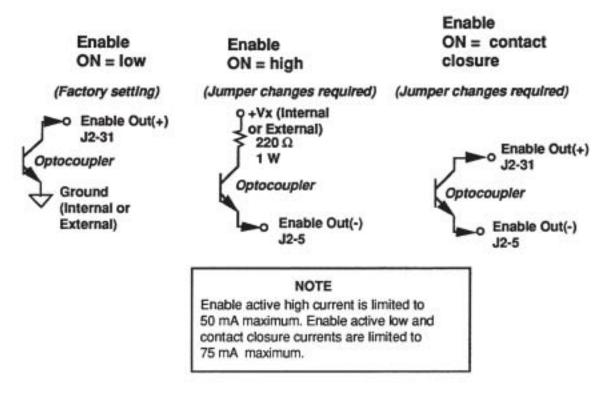
Figure 25-5. Enable Circuit Configurations Changing the Enable Sense
