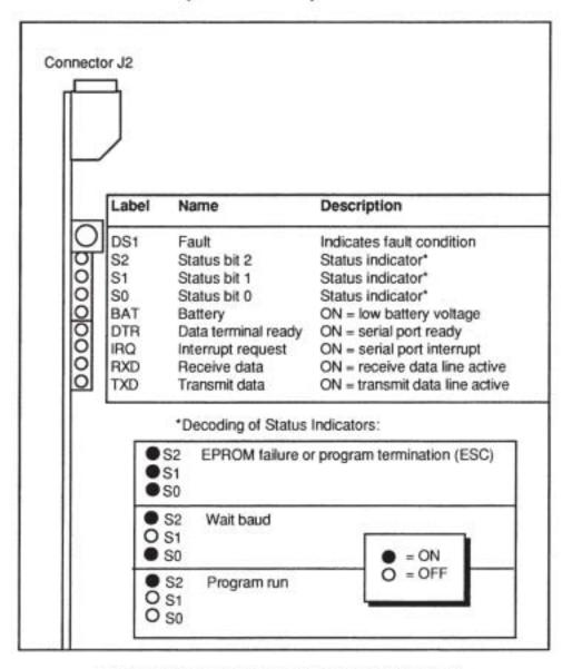
Figure 4-2. System Processor Indicators and Test Points
