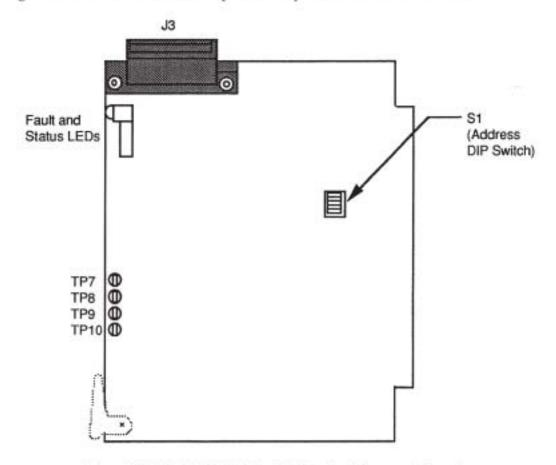
Figure 23-1. Model 473.24c Encoder Interface Component Location
