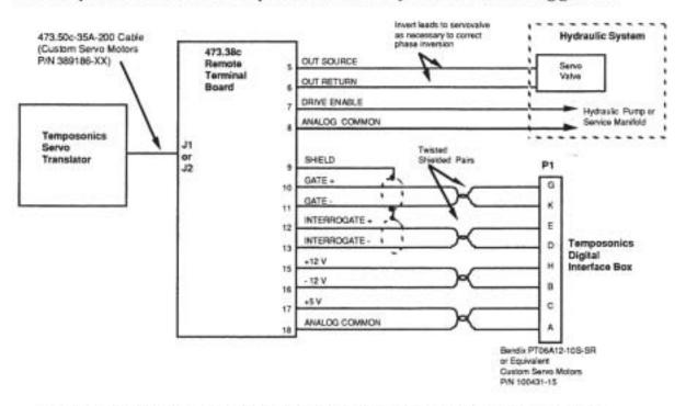
Figure 24-2. Cable Configuration for the Temposonics Servo Translator When Using an Analog Current Velocity Command
