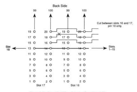
Figure 3-5b. Example of Cuts Between Slots 16 and 17
