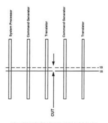
Figure 3-5. Cutting Lines to Isolate Axis Pairs
