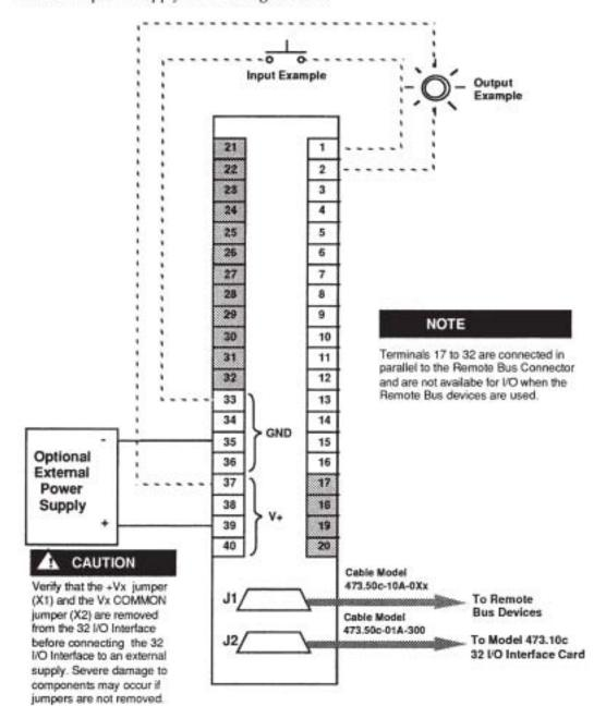
Figure 10-3. Remote Terminal Board to 32 I/O Card
