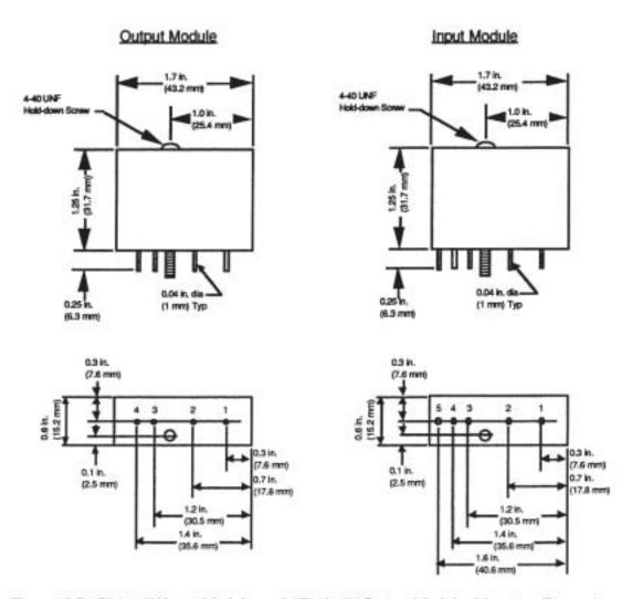
Figure 12-5. 473.11c-0X Input Modules and 473.12c-0X Output Modules Mounting Dimensions
