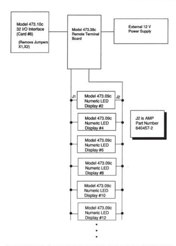
Figure 15-3. Cable Configuration for the Optional External Power Supply With More Than Five Numeric LED Displays
