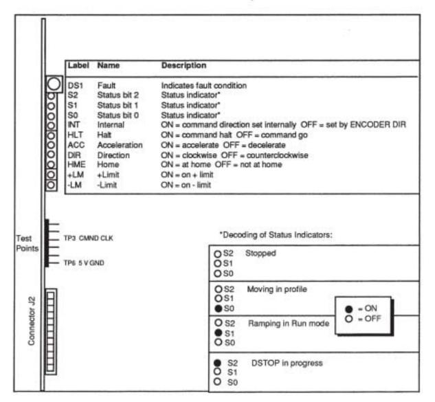
You can use the Fault and Status indicators on the Command Generator/Translator to help in troubleshooting problems which occur when installing the Command Generator/Translator. The status LEDs are in known states during the following operations:
