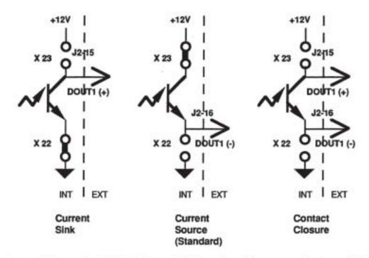
Figure 8-9. Examples of DOUT1 Output Configurations. Current sourcing is standard.
