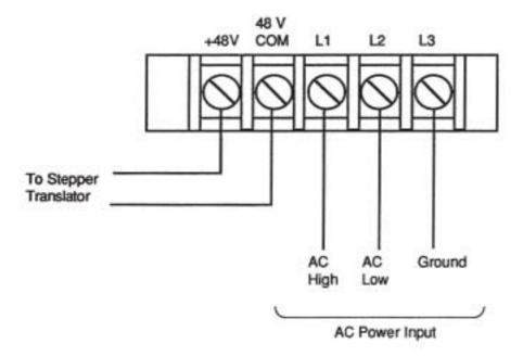
Figure 20-2. Wiring Connections
