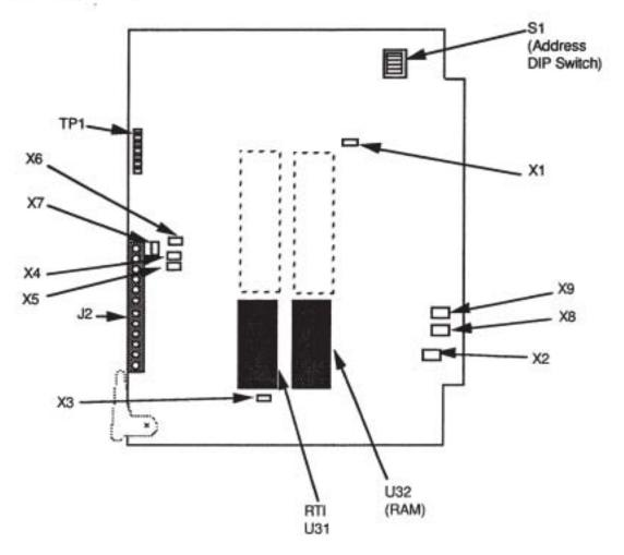
Figure 7-1. Model 473.61c-02A Command Generator/Translator
