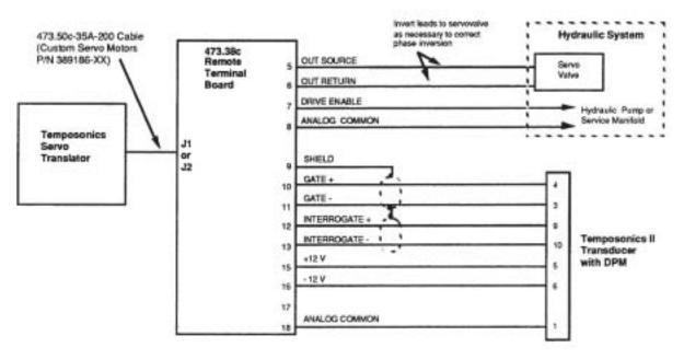
Figure 24-2a. Cable Configuration for the Temposonics II Transducer
