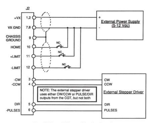
Figure 7-3. Command Generator/Translator Connections
