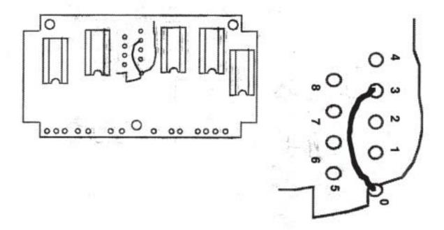
Figure D-6. Example of Recirculation Jumper Setting (0-3 for 4 Recirculations)
