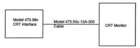
Figure 17-2. Cable Configuration for the CRT Interface
