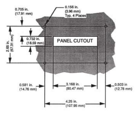
Figure 16-4. 473.13c LCD Display Mounting Dimensions
