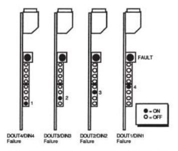
Figure 8-17.LED Indications for the Digital Loop-back Test
