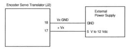
Figure 26-4. External Power Connections
