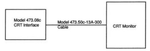
Figure 18-3. Cable Configuration for the 9-inch CRT Display Monitor
