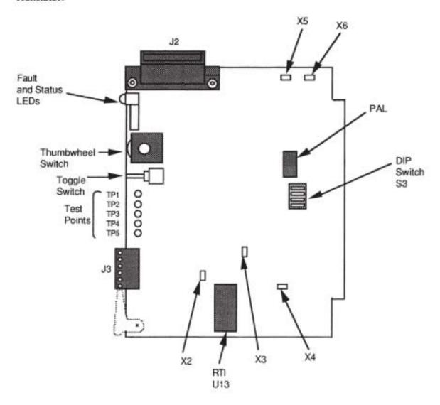
Figure 24-1. Model 473.21c Temposonics Servo Translator Component Location
