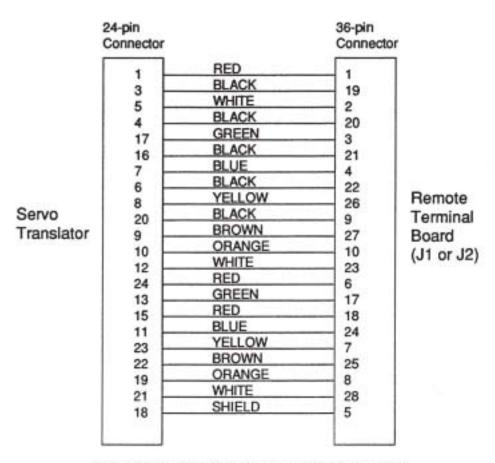
Figure 29-12. Cable Configuration (473.50c-31A-200)
