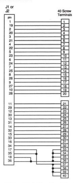
Figure 11-3. Remote Terminal Board Internal Connections
