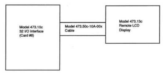
Figure 16-3. Cable Configuration for the Remote LCD Display
