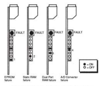
Figure 8-12. LED Fault Indications at Power-up
