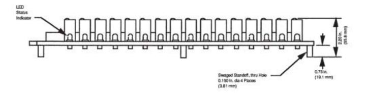
Figure 12-4. 473.36c-0X Motherboard Mounting Dimensions
