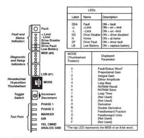
Figure 26-7. Edge-Mounted Switches, Indicators, and Test Points
