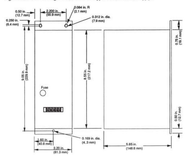
Figure 20-3. Mounting Dimensions
