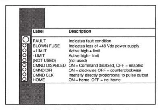
Figure 19-4. Fault and Status Indicator LEDs on the Stepper Translator
