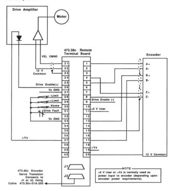
Figure 26-2. Cable Configuration for the Encoder Servo Translator
