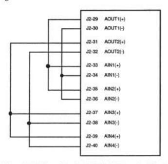
Figure 8-13. Connections for the Analog Loop-back Test
