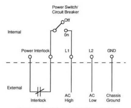
Figure 3-9. Input Power Wiring and Power Interlock
