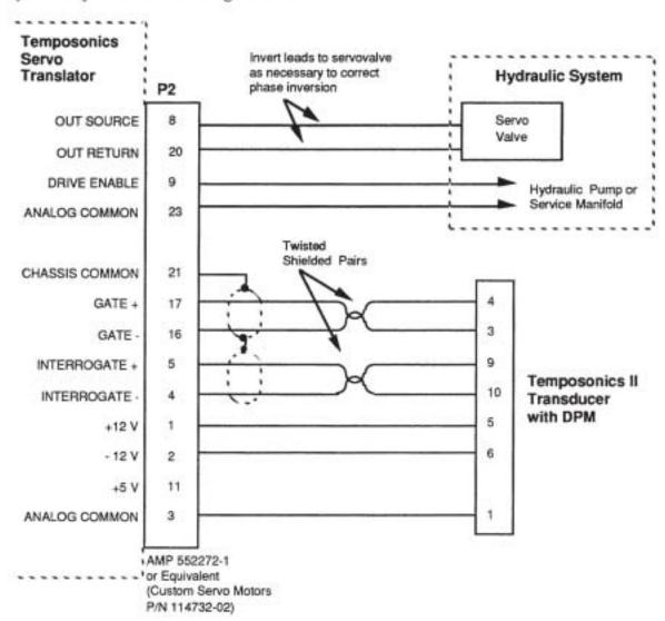
Figure 24-3a. Optional Cabling Example for Temposonics II Transducer When Using an Analog Current Velocity Command
