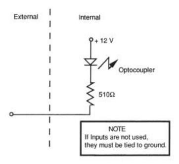
Figure 26-6. Internal Configuration of Limit, Home, and Drive Fault Inputs
