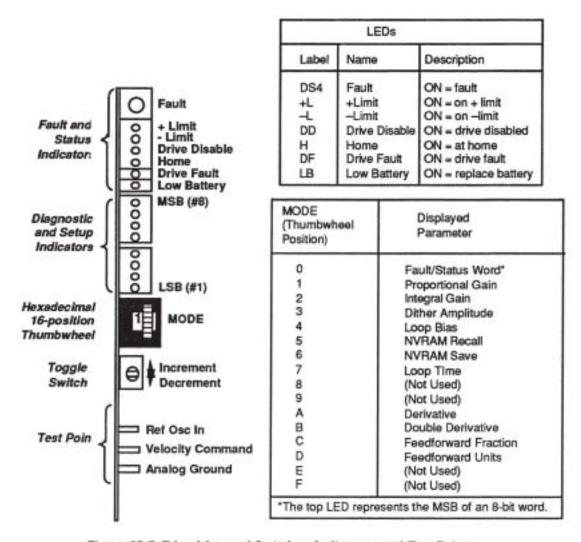
Figure 25-7. Edge-Mounted Switches, Indicators, and Test Points
