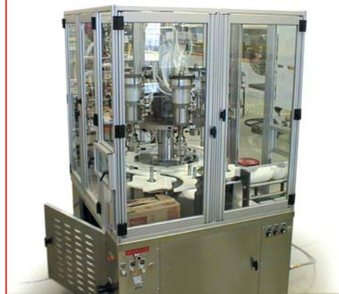
Guarding enclosure using tempered glass
