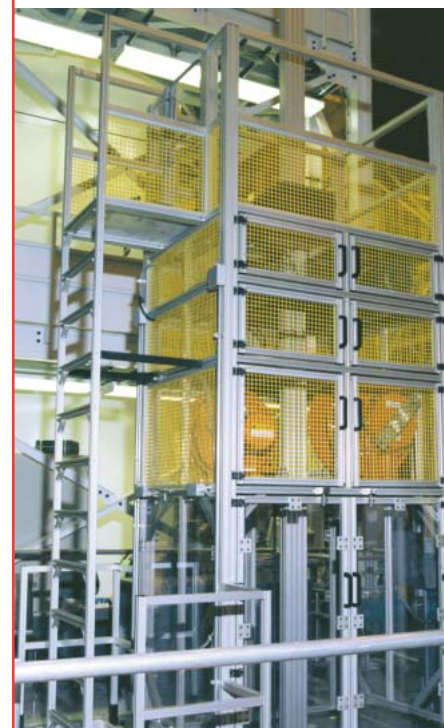
Support structure for drilling apparatus to clean spent fuel remains from space shuttle solid fuel rocket boosters
